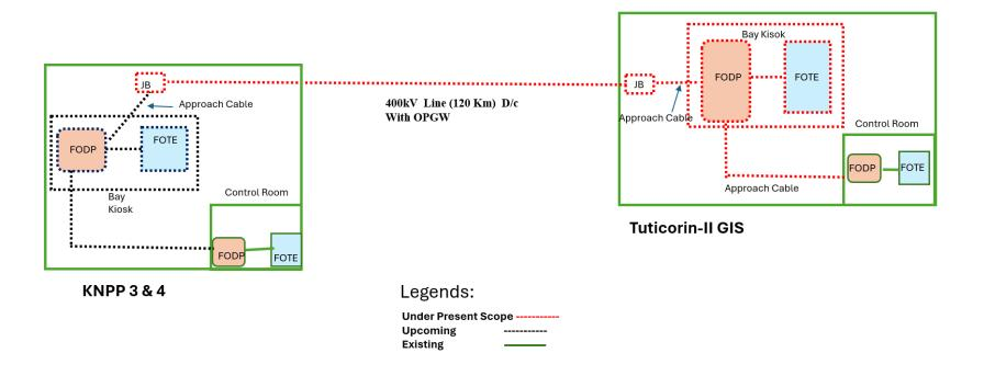
Note: Communication related scope (FOTE/ FODP/ Approach cable etc.) at KNPP 3 & 4 is under NPCIL
