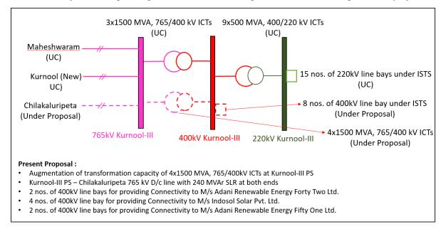
Transmission system strengthening at Kurnool-III PS for integration of additional RE generation projects
