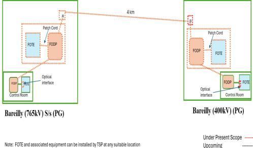
Note: FOTE and associated equipment can be installed by TSP at any suitable location inside S/s premises
