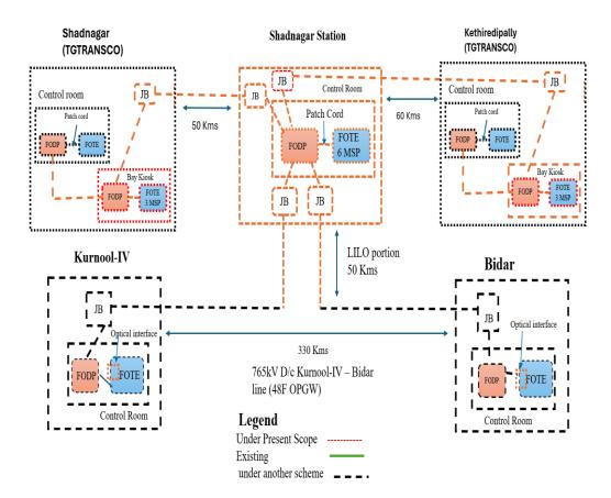
Proposed Communication for "Transmission System for Kurnool-IV REZ - Phase-II (3 GW)"
